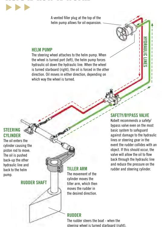
The diagram shows the most basic manual hydraulic system. However, additional helm stations or another rudder can be added to work in multiple configurations. Kobelt will customize the system to work for your specific vessel's needs.
