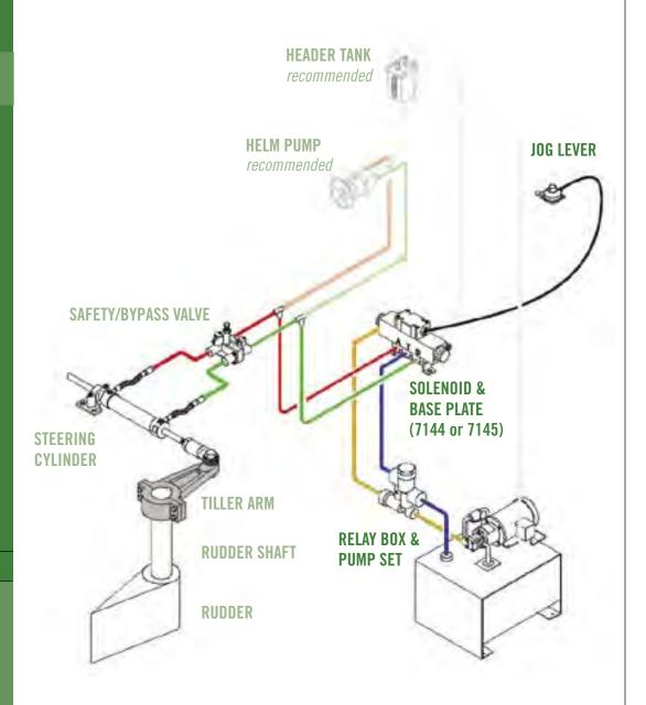
Basic Terms: **Non Follow-Up** refers to a steering system that activates the rudder as long as the jog lever is held to the request. When the jog lever is moved into the "on" position, the rudder begins to turn and continues to turn until the lever is released or it reaches the limit of its operation.
